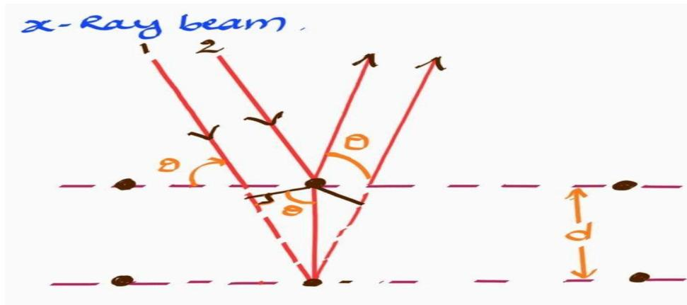
**Analysis:** XRD analysis is based on Bragg's Law and Bragg's angle.
