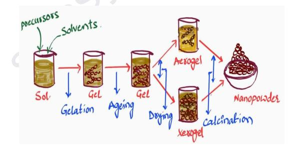
(**i)** Formation Sol : Take precursors(raw material) like metal alkoxide or metal salts and dissolved in water or alcohol or other solvents.
