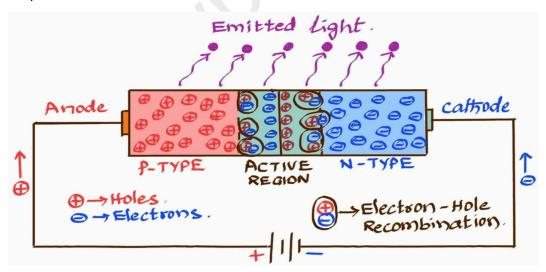
The energy of light radiation depends on the strength of the recombination and the materials used. The emitted light is very small in intensity and is of the order of the microampere range. The energy released in the form of a photon is equal to the forbidden energy gap (Eg) and is equal to hv
