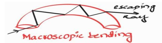
To prevent macrobends, optical fiber has a minimum bend radius specification that should not be exceeded.
