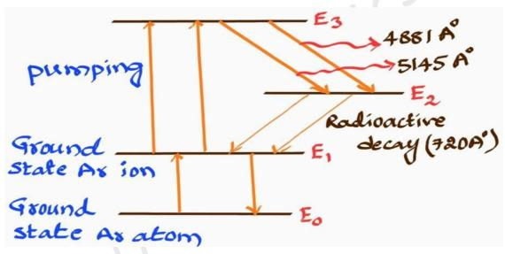
The energy level diagram of Ar-ion Laser is shown below.
